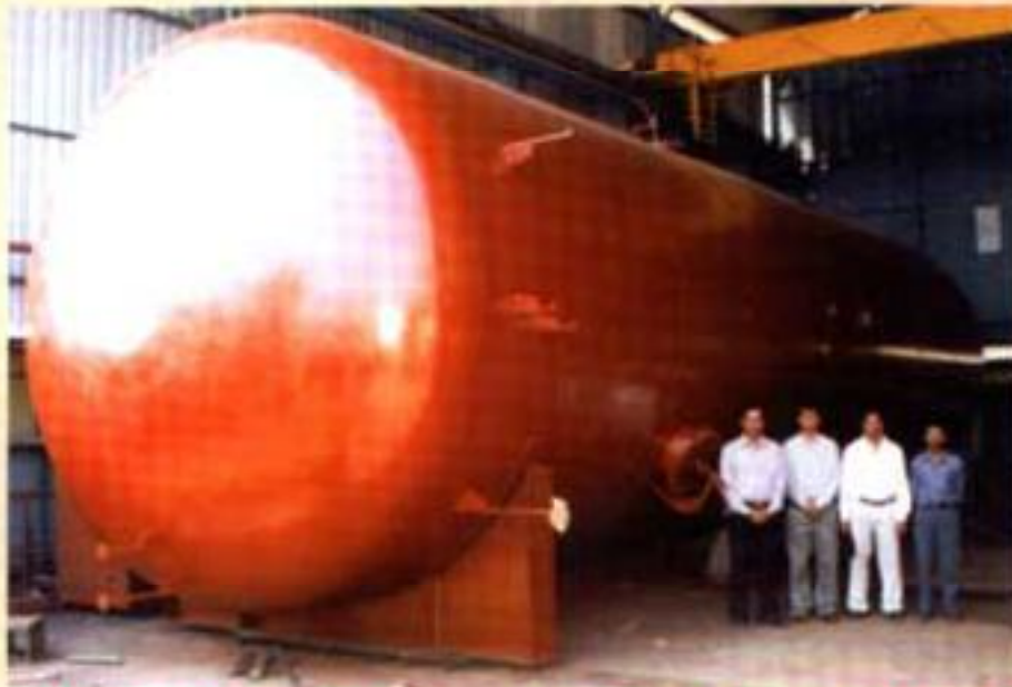
4 MTR DIA X 13 MTR LONG SINGLE PIECE 20 TONS DEAERATOR
